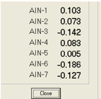
If you do wish to use the additional analog inputs, you can display them by selecting “Show analog inputs” from the Setup menu on the IO Status window. You can also access these inputs using the command ?AIN, where *n* is a number between 0 and 7.
