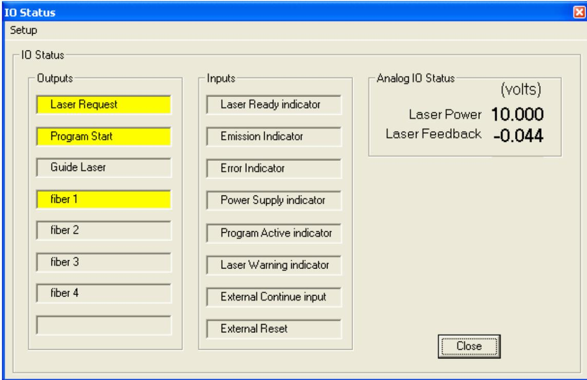
This shows the current input and output status of the IPGpulser. The Laser Power and Laser Feedback fields show the current analog values generated and monitored by the system. **Note:** the Laser Power is the value that was sent to the D/A output on the system, not the actual measured voltage at that output. You can edit the names of the inputs or outputs in the tables by simply clicking and typing. Typically, you may wish to rename the fiber outputs as real workstation names.
