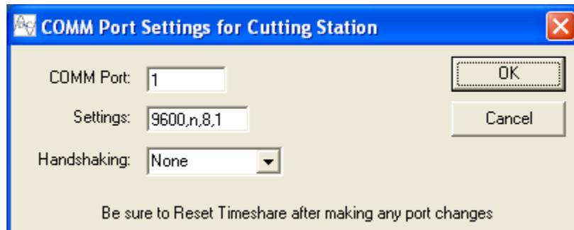
**Note:** The communications used between the IPGpulser and CNC systems consists of very short conversations. The use of hardware handshaking will probably have no effect on performance. Increasing your baud rate to its maximum while still maintaining a reliable connection will provide better performance.
